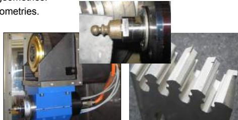
Fir-tree slots in a nickel alloy ground with a form electroplated CBN wheel of diameter of about 4 – 15 mm. A high speed spindle attachment (75,000 rpm) was used to drive the small wheel.
