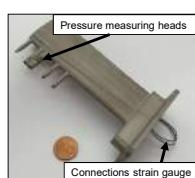
Fig. 1: Rake of the company Vectoflow with integrated strain gauge
