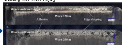
(a) Wear on the rake face after 128 m (wear condition I);
