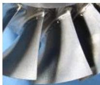
A nickel alloy integral bladed rotor (IBR) machined by 5-axis grinding with an electroplated CBN wheel of 10 mm diameter [4].
