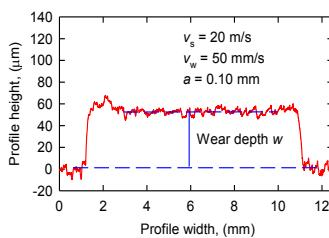
Measured radial wheel wear profile
