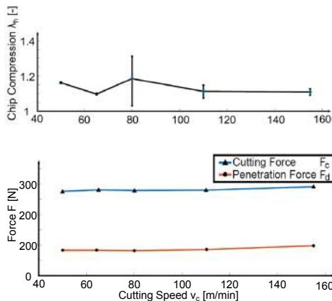
**Tool:** HW-K10, CNGP 120408,  $\alpha_{\text{eff}} = 6^\circ$ ,  $\gamma_{\text{eff}} = 2^\circ$ ,  $k_r = 95^\circ$ ,  $r_\beta = 6+2 \mu\text{m}$
