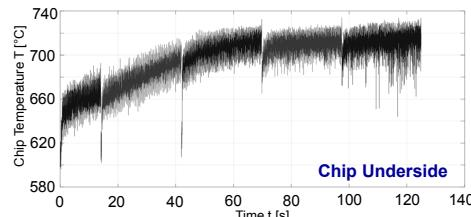
Tool: HW-K10, CNGP 120408,  $\alpha_{\text{eff}} = 6^\circ$ ,  $V_{\text{eff}} = 2^\circ$ ,  $\kappa_r = 95^\circ$ ,  $r_\beta = 6+2 \mu\text{m}$
