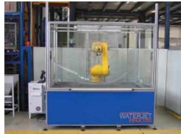
Waterjet HRX 160 with six-axis robot manipulator
