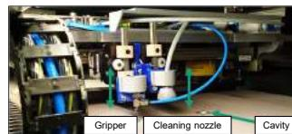
Fig. 2: Automation unit for sensor integration
