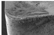
Cutting edge when machining titanium alloys [1].
