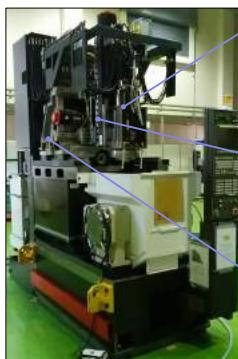
**Main spindle** CFRP with steel sleeve
