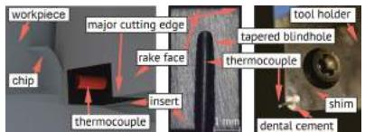
Measurement of the tool temperature at a distance of 1 mm to the contact zone.
