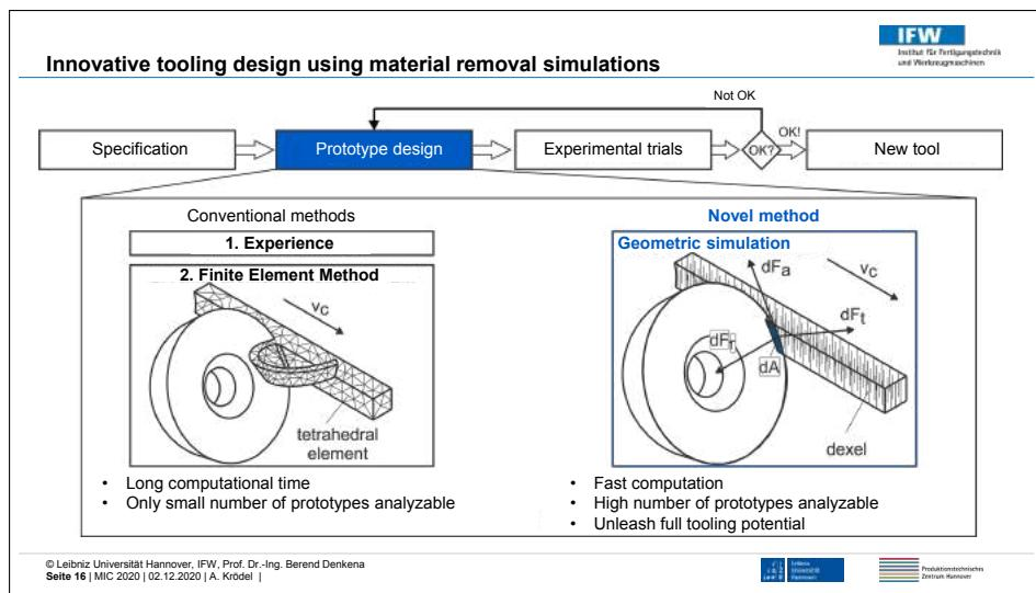
**Example: Simulation based design of a novel porcupine milling cutter**
