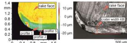
Methodology of the crater wear measurement of the cutting tool using structured-light 3D scanner (left) and optical microscope (right).
