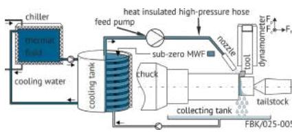
Sub-zero MWF supplying system integrated in the lathe.
