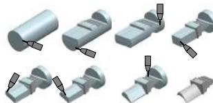
Trimming of a turbine blade using AWIJC
