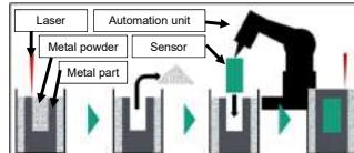
Fig. 1: Concept for sensor integration
