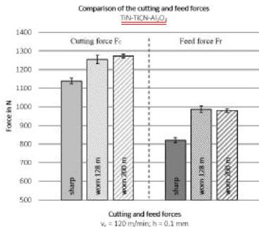
Conclusion: The pre-wear of the inserts leads to an increase in the cutting and feed force. The multilayer coating TiN-TiCN-Al<sub>2</sub>O<sub>3</sub> tends to higher feed forces.
