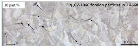
Foreign particles remaining in the powder material after reconditioning can lead to structural defects.
