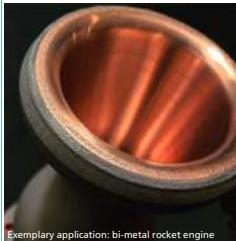
Exemplary application: bi-metal rocket engine produced via Directed Energy Deposition by Launcher<sup>1</sup>
