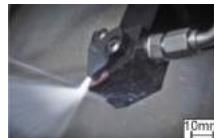
Dual coolant supply on flank and rake surface in the context of turning [2].
