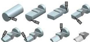
Trimming of a turbine blade using AWIJC
