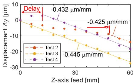
Y-axis error according to Z-axis feed is  $-0.434 \mu\text{m}/\text{mm}$  ( $-24.9 \times 10^{-3} \text{ deg}$ )
